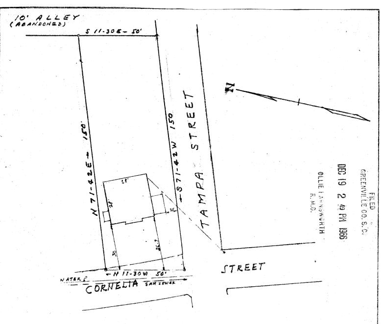
This is to certify that on Dec. 9, 1966, I surveyed the property shown on this plat, and that the property lines, walls and building are as shown hereon; that the building located on said lot does not encroach or project on adjacent streets or property, and that no adjacent walls or building encroach or project on said premises, and that no utility lines cross this property except as shown hereon.
