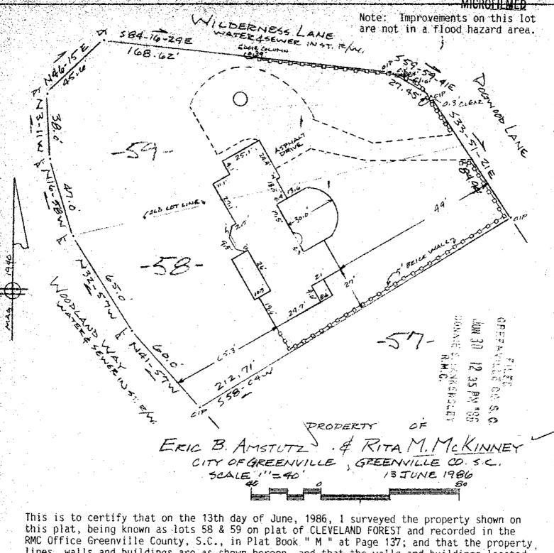
lines, walls and buildings are as shown hereon, and that the walls and buildings located on said lot do not encroach or project on adjacent street or property, and that no adjacent walls or buildings encroach or project on said premises, no power lines cross this property and no visible encroachments except as shown hereon.
