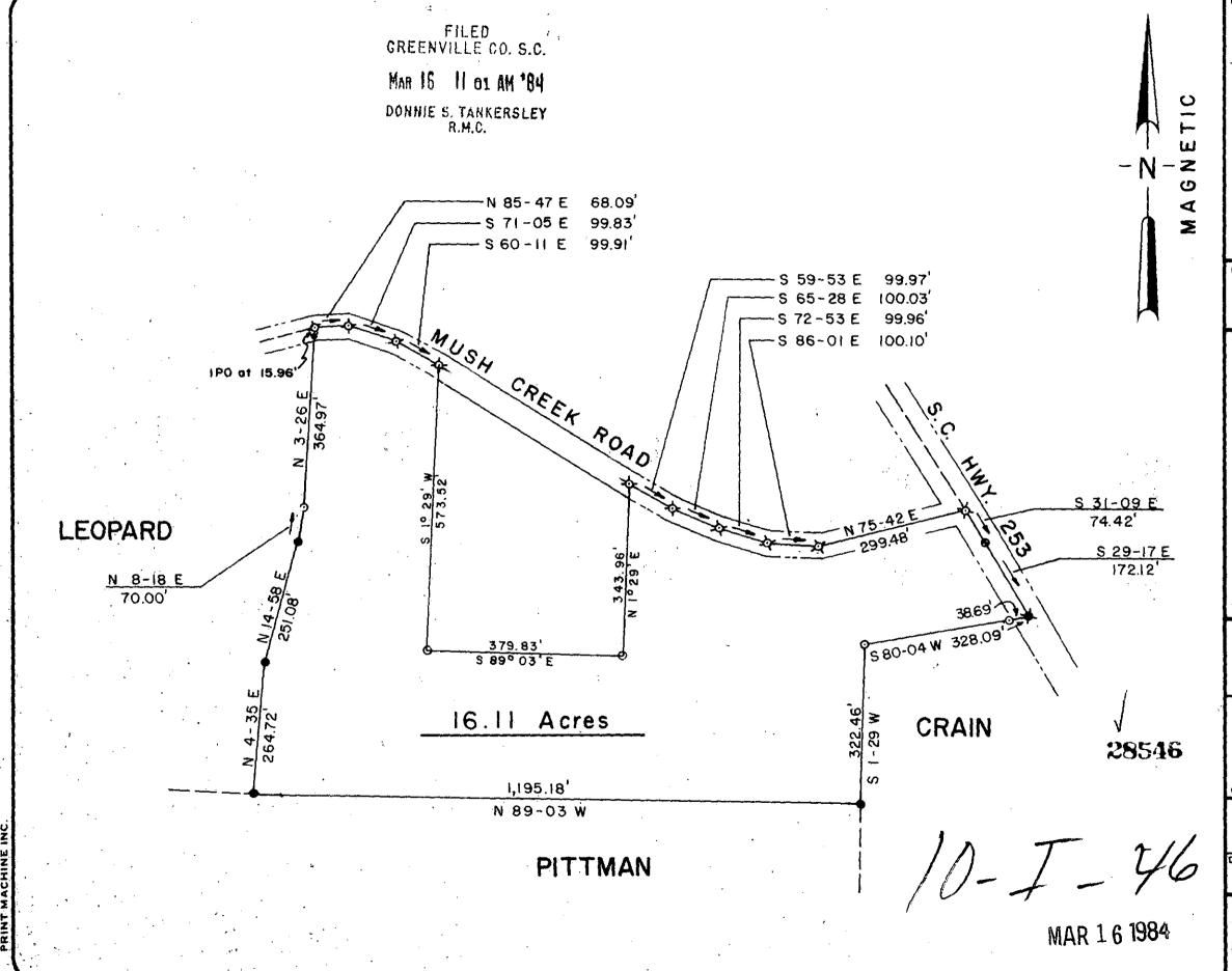
0 I.P. SET STONE R.R. SPIKE I.P. FOUND NAIL & CAP NAIL / CAP FOUND 🖾 I hereby certify that the ratio of precision of the field survey is 1/10,000 as shown hereon and the area was determined by the coordinate method of area calculation. 1 hereby certify that the measurements as shown on this plat
