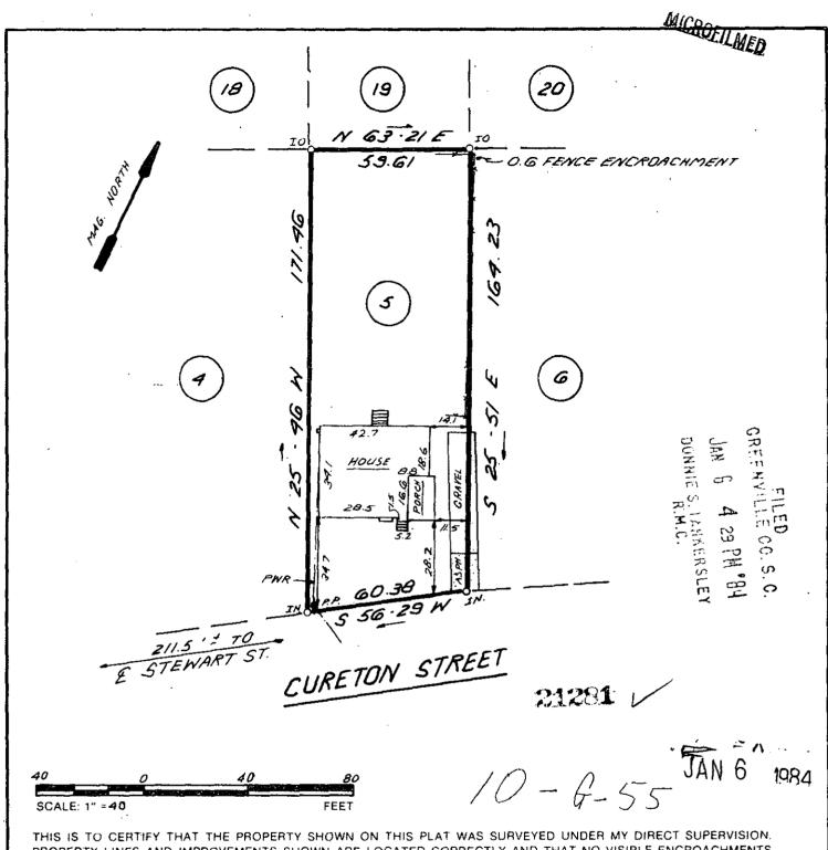
PROPERTY LINES AND IMPROVEMENTS SHOWN ARE LOCATED CORRECTLY AND THAT NO VISIBLE ENCROACHMENTS EXIST UNLESS OTHERWISE SHOWN: THIS PROPERTY IS NOT LOCATED IN A DESIGNATED FLOOD HAZARD AREA.
