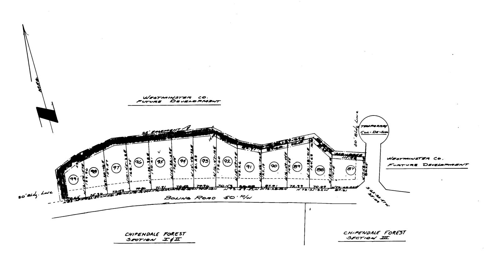
Nort: E' UTILITY & DARINAGE ENGENEMT. ALONG ENCH SIDE | RAME LOT LINES IN MODITION TO BASEMENTS SHOWN ON PLATE ALL LOT CORNERS STAKED WITH IRON PINS.
